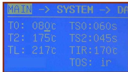
Pressing “UP” or “DOWN” key to change the value of the 1’s digit as“5”, and then pressing “LEFT” key to make the cursor move forwards one digit. Pressing “UP” or “DOWN” key again to change the ten’s digit “9”.
