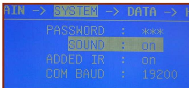
4) Press “SAVE” key to save the data and press “DOWN” key to setting controlling switch state of the out side parts of the infrared heating tubes. If setting “ADDED IR” as “ON”, it means the out side parts of the infrared heating tubes are heating when the bottom heating. Setting method as above.
