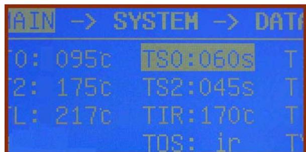
Press “SAVE” key to save the data. Press the “SAVE” again to exit the parameter setting state if only need to set the “TO” and then press “RIGHT” key to the next parameter setting.
