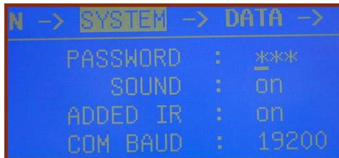
\* Initial password is “000”and omnipotent password is “159”. Users can input omnipotent password “159” if forgetting the setting password and then the system is back to initial password “000”.
