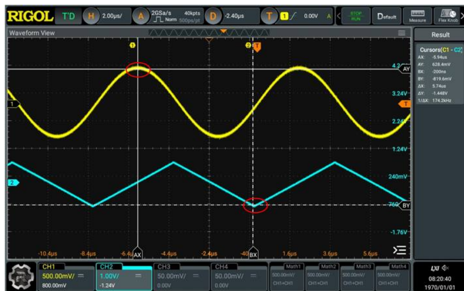
Figure 10.13 Track Measurement (after Horizontal Expansion)
