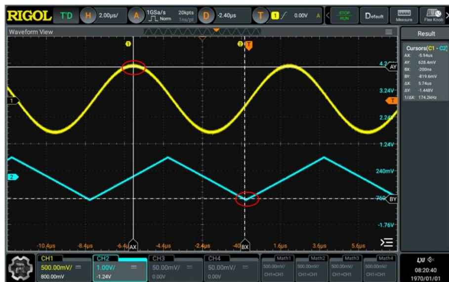
Figure 10.13 Track Measurement (after Horizontal Expansion)
