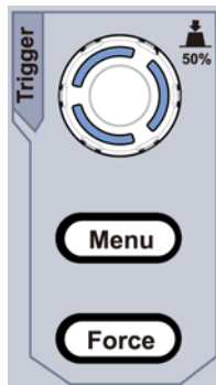
Figure 3-12 Trigger Control Zone
