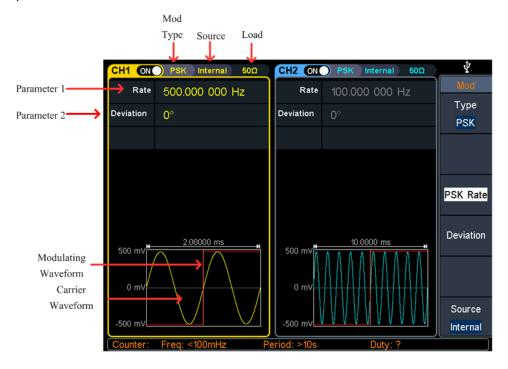
Figure 5-16 Phase shift keying user interface
