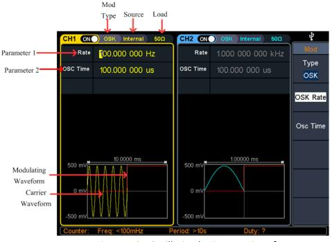
Figure 5-21 Oscillating keying user interface
