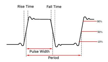
The settable range of pulse width is limited by the "minimum pulse width" and "pulse period"
