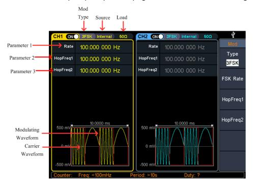
Figure 5-18 Hexadecimal frequency shift keying user interface
