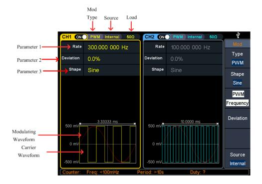
Figure 5-14 Pulse width modulation user interface
