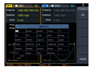
(3) Turn the **knob** to select the desired waveform, for example, select Airy. Press the **OK** soft key to enter the Airy function.
