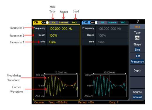
Figure 5-11: Amplitude modulation user interface
