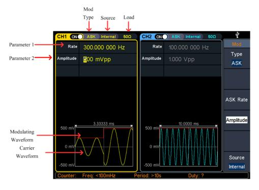
Figure 5-15 Amplitude shift keying user interface
