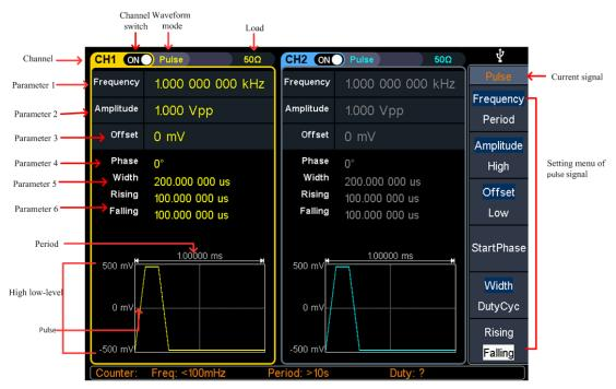
Figure 5-6: Pulse wave user interface
