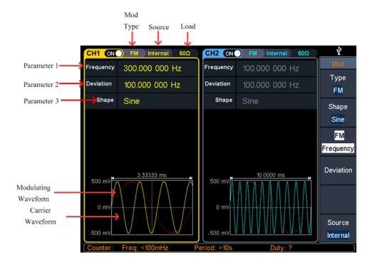
Figure 5-12: frequency modulation user interface
