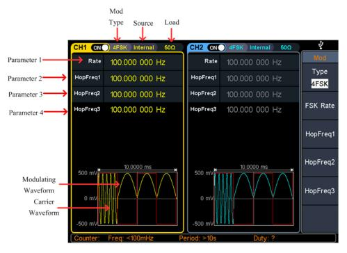
Figure 5-19 Quaternary frequency shift keying user interface
