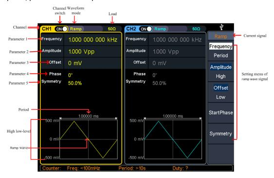
Figure 5-4: Ramp wave user interface
