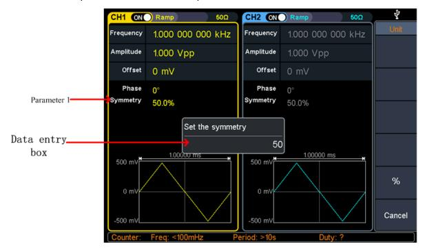
Figure 5-5: Set the symmetry of ramp wave
