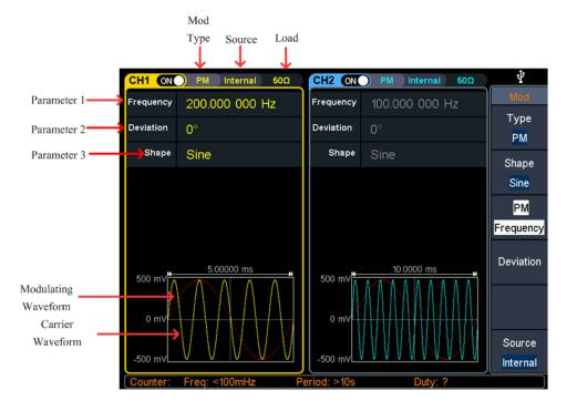
Figure 5-13: Phase modulation user interface
