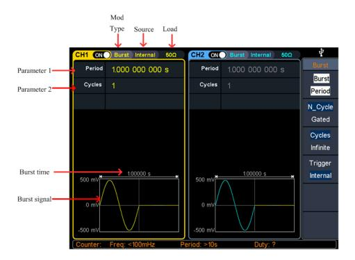
Figure 5-23: N cycle burst user interface
