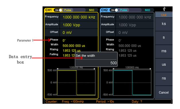
Figure 5-7: Set the pulse width
