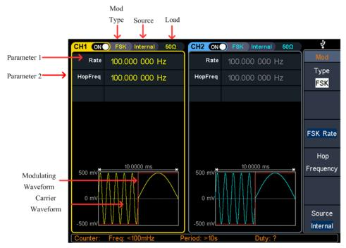
Figure 5-17: Frequency shift keying user interface
